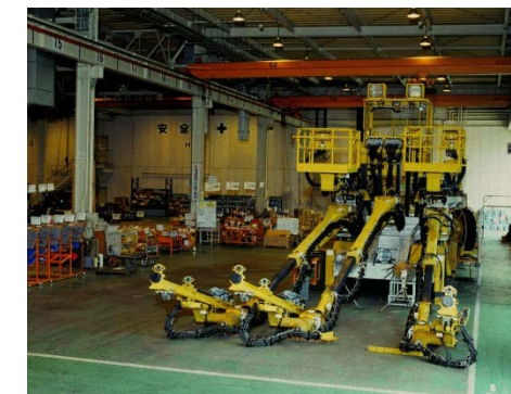
Drill jumbo assembly line
